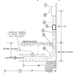
Excavation for foundation must be backfilled and tamped by customer prior to conduit installation to prevent further settling.
